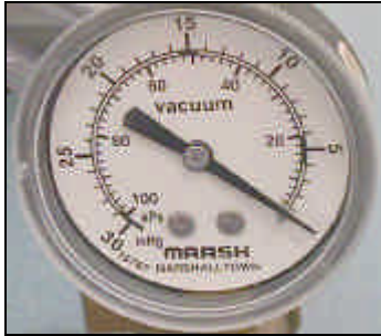
Vacuum gauge reading atmospheric pressure
