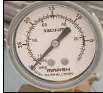
Vacuum gauge reading vacuum (30 inches Hg)
